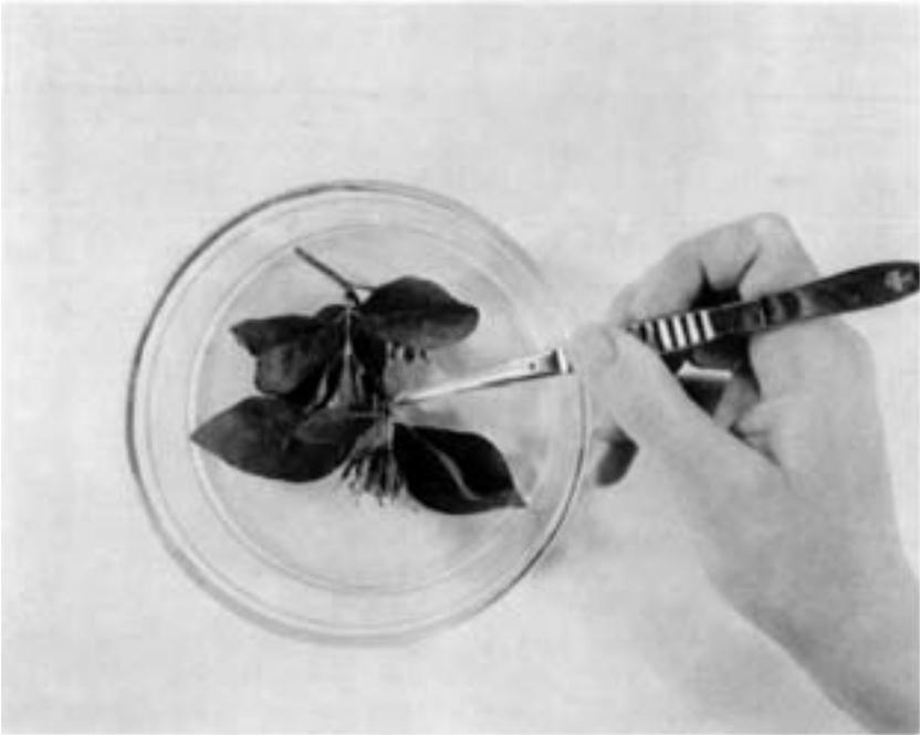
*Positioning a specimen on base layer of plastic.*
