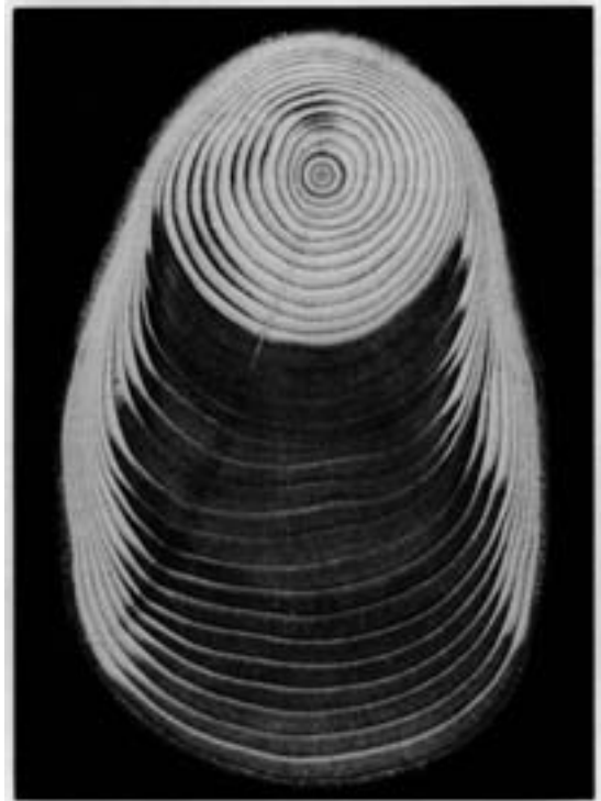
Compression wood in Abies balsamea, the balsam fir, produced along the underside of a leaning trunk, pushing it up into a vertical position. Note the eccentric radial growth caused by the production of darkly stained compression wood on the lower portion of the cross section. Photo by T. E. Timell.
